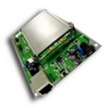
The EZBridge PCB card aims at providing assistance in building a connection between your wired LAN and one or more Wireless Local Area Networks.
