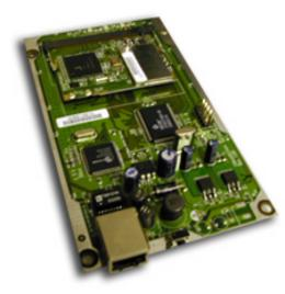
The EZBridge PCB card aims at providing assistance in building a high-speed connection between your wired LAN and one or more Wireless Local Area Networks.
