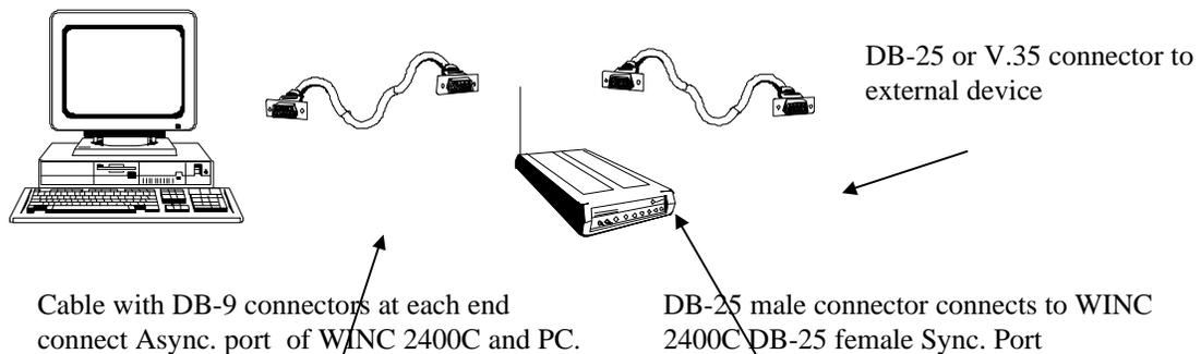
**Fig. 4.0 Wiring Interface**
