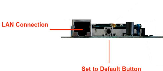
**LAN Connection** Use Ethernet straight LAN cable to connect your PC, hub/switch or broadband router/modem to this port.
