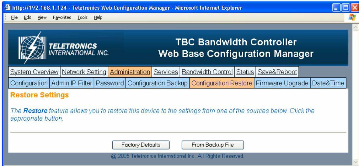
This section allows the bandwidth controller to restore default factory settings by clicking Factory Defaults, or to restore from a backup configuration file (the .tar file) to a previous setting point by clicking From Backup File.
