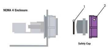
Re-using items (1) and (2) from the safety cap, assemble the waterproof RJ-45 connector as shown below:
