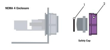
Re-using items (1) and (2) from the safety cap, assemble the waterproof RJ-45 connector as shown below:
