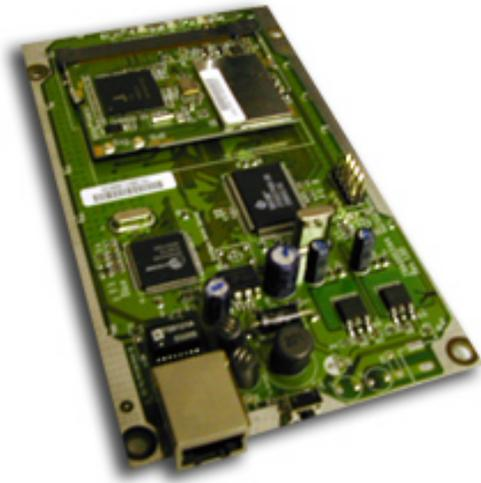
The EZBridge PCB card aims at providing assistance in building a high-speed connection between your wired LAN and one or more Wireless Local Area Networks.
